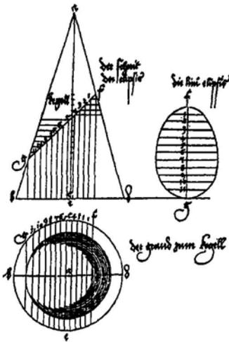
**Figure 5.4: Whether a section of a cone is the same as a section of a cylinder, and whether either is egg-shaped, has long been debated. Here Dürer's discussion of the ellipse (Underweysung der Messung, 1525)**
