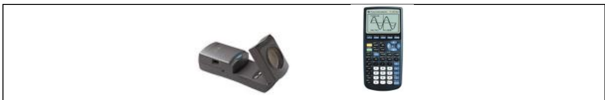
Figure 4. The Based Ranger Calculator ® (to the left) is an artefact conceived of in order to study objects in movement: through the emission of waves, the CBR collects data about the distance from it to the object in question. When it connects to a graphic calculator (for example, the TI-83+ ® , shown on the right), it is possible to get graphics such as space-time, velocity-time, etc.
